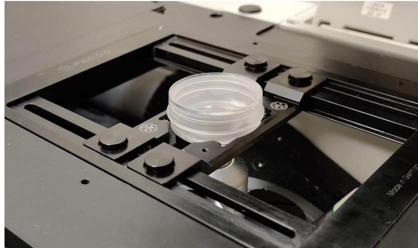
These are [inverted microscopes](#) with the objectives below the specimen. If using a slide with attached coverslip, you must turn it [upside down](#) to image.
