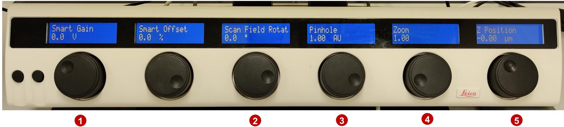
The controller panel allows to change some of the parameter for image acquisition. All settings can also be made in the software. The standard configuration is:
