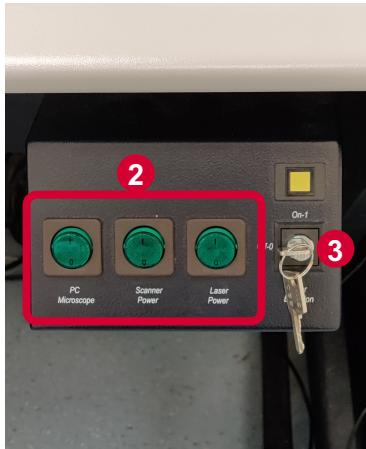
When the computer is off, turn off **Laser Power**, **Scanner Power Switches**, and **PC Microscope** (② green switches) then turn **Laser Key** ③ to off state.
