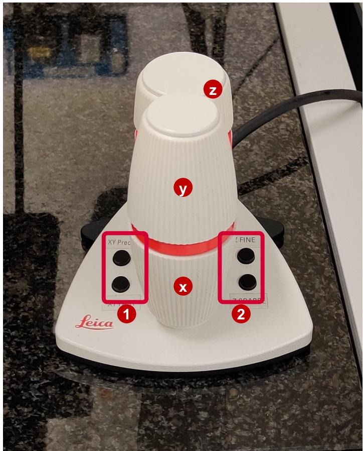
To move the stage in the X/Y/Z plane, the ‘salt and pepper’ controller can be used.
