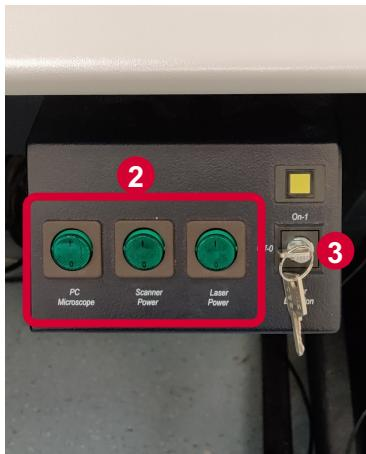
Turn on Laser Power, Scanner Power Switches, and PC Microscope (② green switches) then turn Laser Key ③ to on state.
