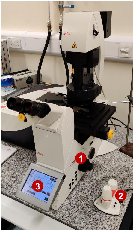
The microscope frame is equipped with standard controls like **focusing knobs** ① on the left and right side of the stand
