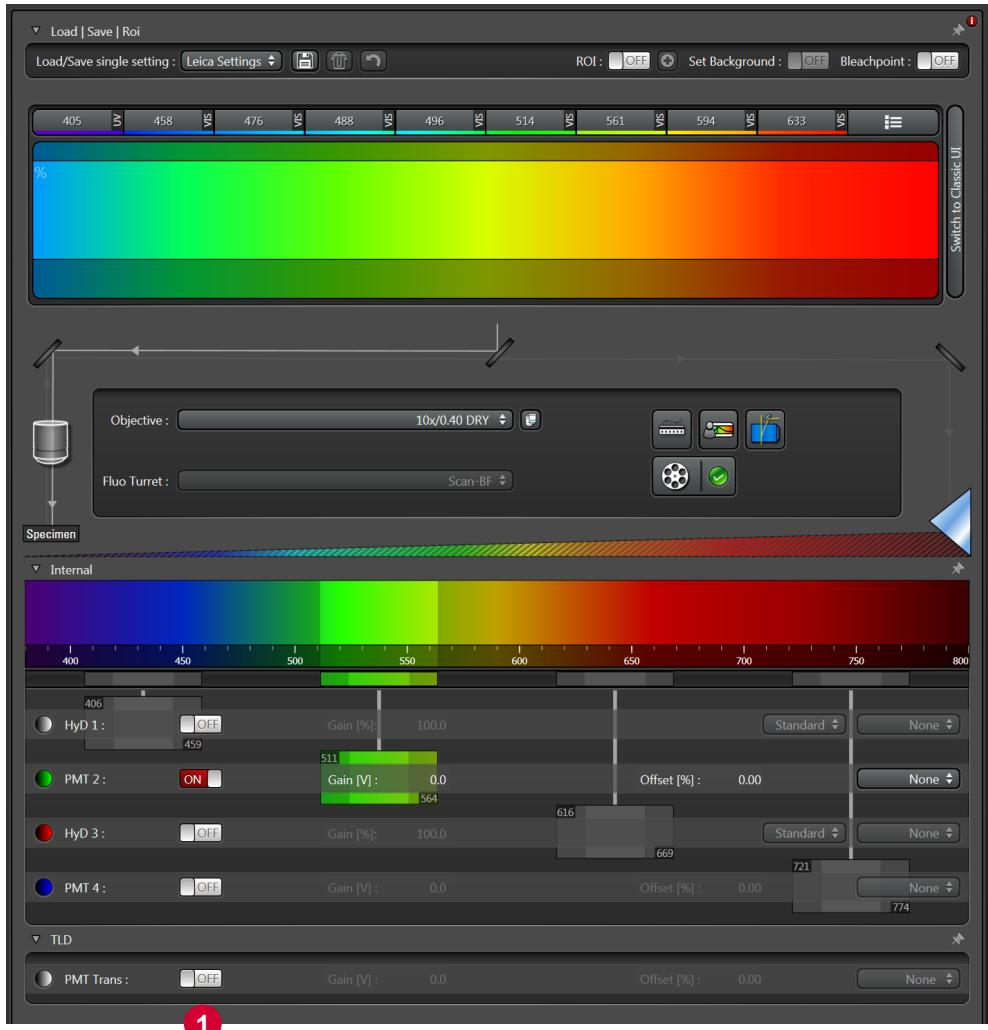
To add a **transmitted light image** to your acquisition turn on the **PMT Trans detector** ① in one of your sequences.
