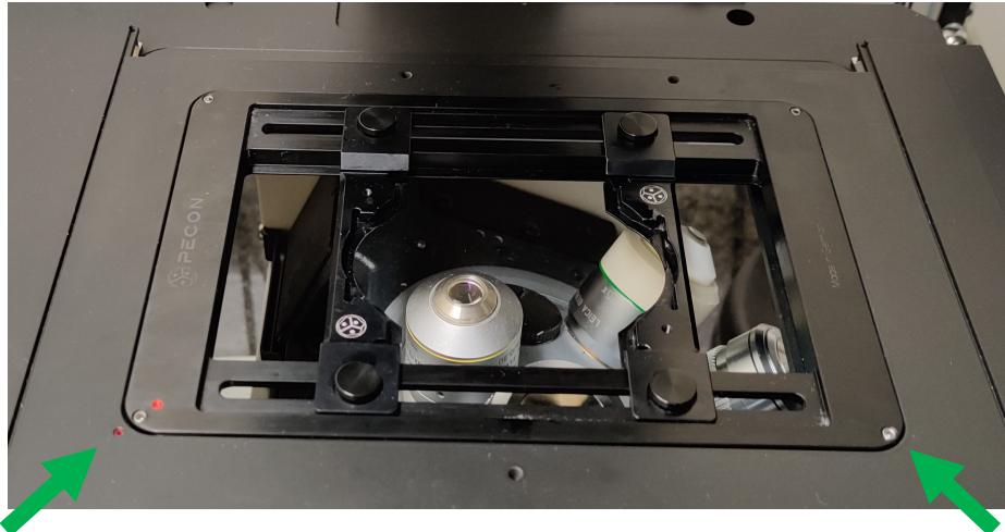
Make sure the stage insert is correctly inserted and sitting flat
